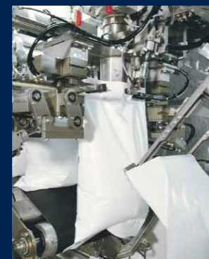
HAYER FFS liquid bag at the filling spout
